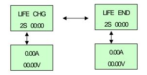
a. When a Charge (CHG) mode **WITH** balancer connected is finished, screens as below appear at charge finish (LiFePO4 example).
