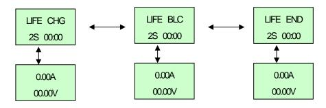
a. When a Balance-Only (BLC) mode is finished, screens as below appear at balance finish (LiFePO4 example).
