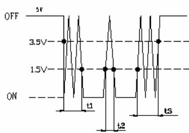
( $t_1, t_3$ ) : Masking time to avoid chattering.
