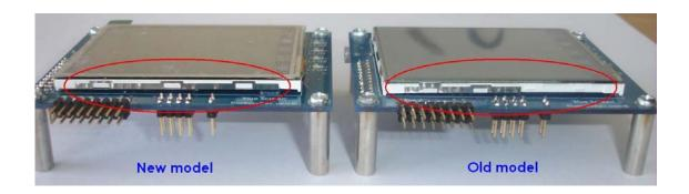
These two models have a major different on the LCD controller. The old one, ELT240320TP comes with ILI9320 and the new one, ELT240320ATP comes with ILI9325. The only change on software in the example code is its initial codes. Anyway, in order to supply the codes which support both models of LCD, the driver code has to be read before sending those initial commands. The initial function, TSLCDInit() is modified.
