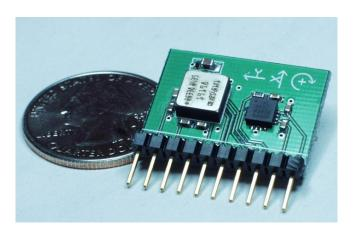
2 Degree of Freedom Gyroscope/ Accelerometer Combination 11/13/2004
