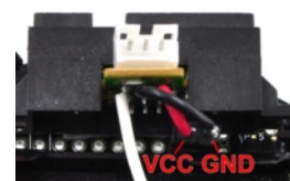
Connections for the 3pi wall follower's 1×2 header.
