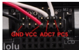
Connections for 3pi wall follower's 2×7 header.
