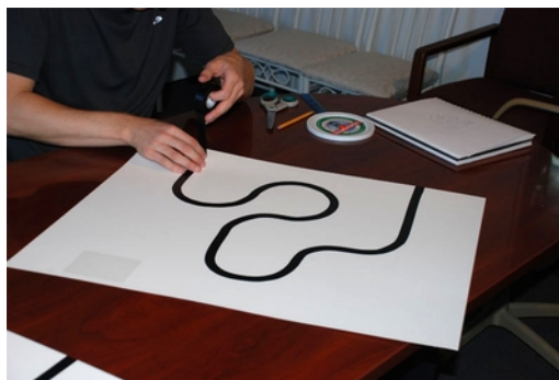
Construct the second half of the line course in the same way.
