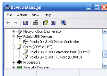
Windows XP device manager showing the Pololu Jrk 21v3 Motor Controller
