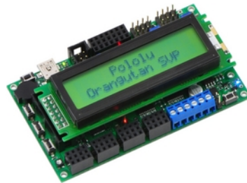
Orangutan SVP fully assembled.
