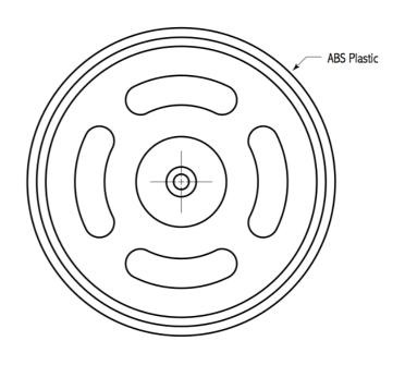
Rubber band tires increase wheel diameter to 67mm
