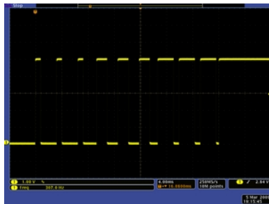
Qik 2s12v10 motor driving from speed 0 to 127 with acceleration of 127 and PWM frequency of 310 Hz.
