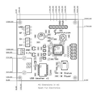
The USB Weather Board is relatively straight forward in operation. The unit can be powered through USB or a separate 4-7V header with an on/off switch for easy power on/off.
