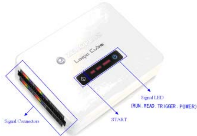
Fig. 1-9: A View of the ZeroPlus Logic Analyzer LAP-C Series. See Fig 1-11 for detailed information on the Signal Connectors
